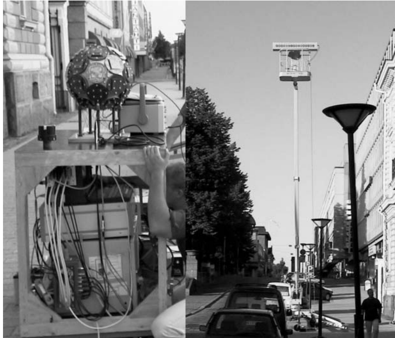
Figure 6.36 HUT MIMO measurements TX (left) and RX (right) in a microcell [KSPH01].
